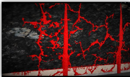
SwellFrac Fully Swelled Plugging off the Frac Matrix
